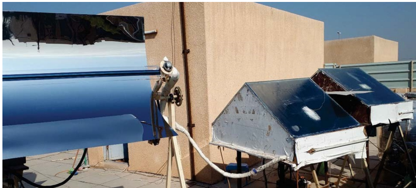
Fig. 1. DSSD with Parabolic Collector Integrated with PCM
