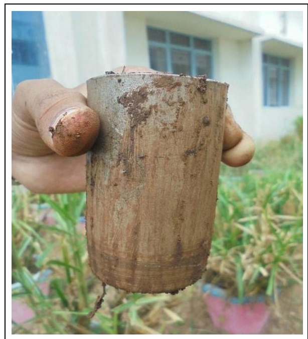
Fig. 4: An undisturbed soil sample taken from the pot
