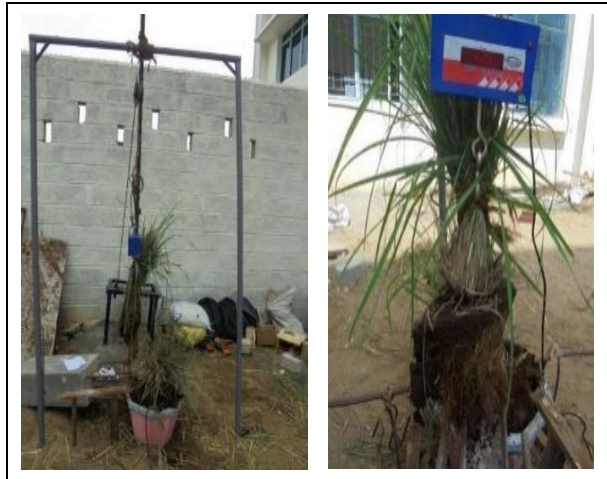
Fig. 5: The Pull-Out resistance test for the lemon grass plant
