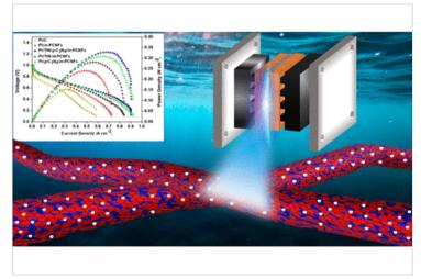
C<sub>3</sub>N<sub>4</sub> and Ti-N-C moieties provides strong metal support interactions to the catalyst layer on the MEA, facilitating ORR activity and stability. The surface-engineered Pt/TiN/q-C<sub>3</sub>N<sub>4</sub>/m-PCNFs exhibited outstanding electrocatalytic performance (electrochemical surface area (ECSA) = 95  $m^2/g$ ) compared to commercial Pt/C
