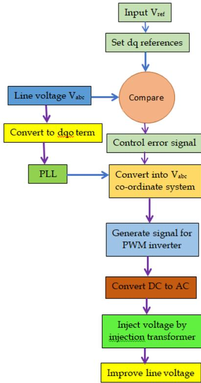
**Figure 7:** Operation of DVR under voltage deviations
