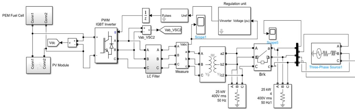
Figure 5: MATLAB/Simulink model of Solar PV-PEMFC Hybrid Energy System
