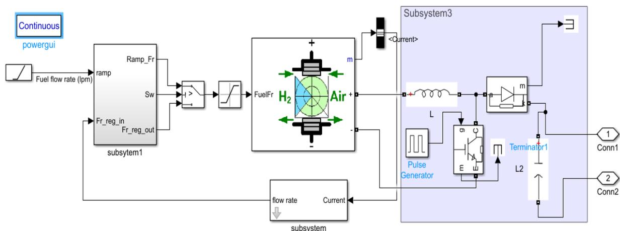
Figure 4: MATLAB/Simulink model of PEMFC
