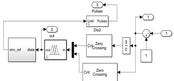
**Figure 9:** Fuzzy logic-based DVR control circuit
