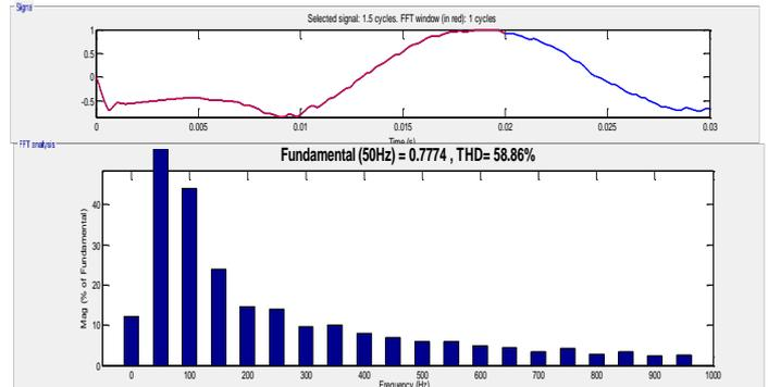
**Figure 13:** Frequency spectrum of output voltage with DVR
