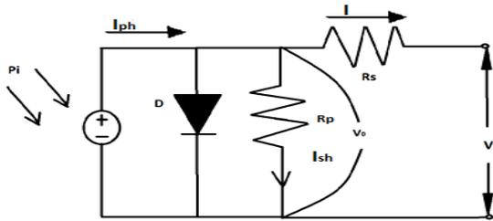
Figure 2: Solar PV cell Model
