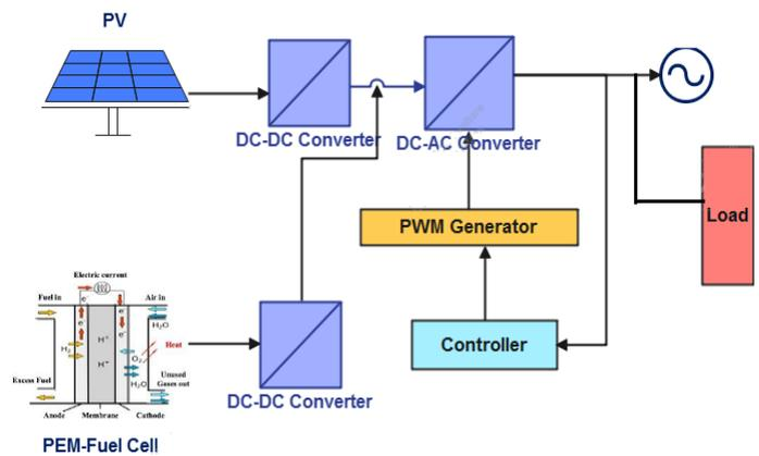
**Figure 1:** Proposed Hybrid Energy System with Solar PV and PEMFC
