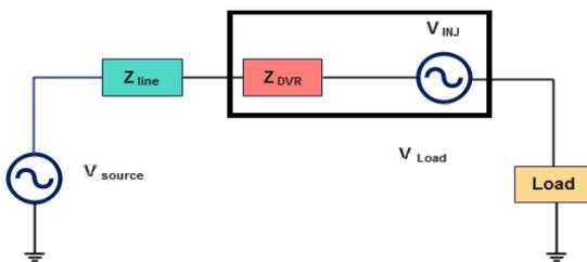
Figure 6: Equivalent structure of DVR
