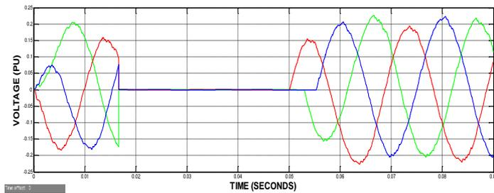
**Figure 10:** Waveform of the HES's output voltage without the DVR
