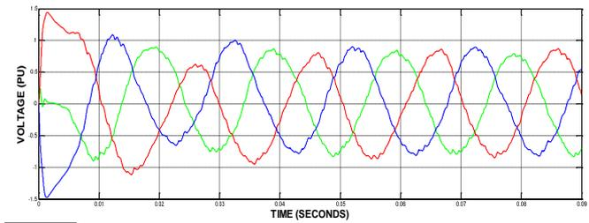
**Figure 14:** HES output voltage waveform with FCDVR
