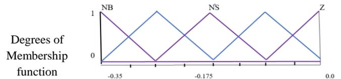
**Figure 8:** Input membership function for fuzzy logic controller
