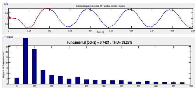
**Figure 15:** Frequency spectrum of output voltage with FCDVR
