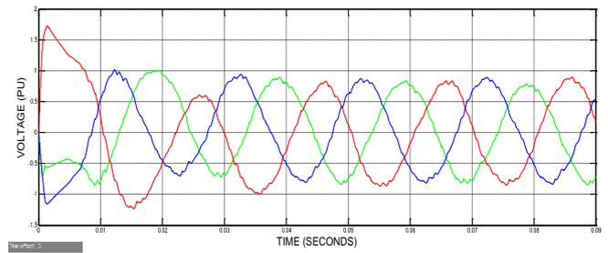
**Figure 12:** HES output voltage waveform with DVR
