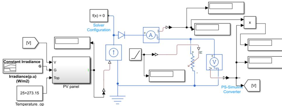
Figure 3: MATLAB/Simulink model of solar PV system
