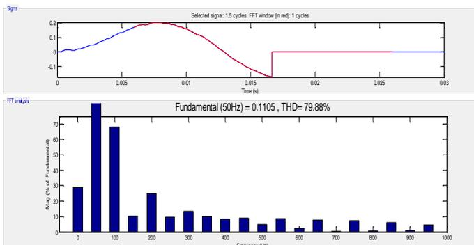
**Figure 11:** Output voltage frequency spectrum without DVR
