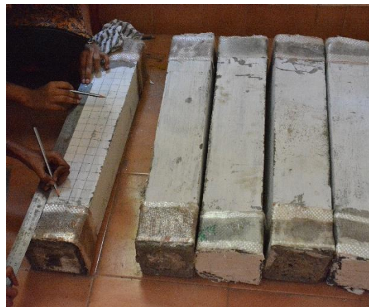
Figure 2. Columns prepared for testing.
