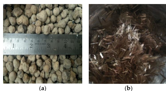
Figure 1. Details of the materials used. (a) Sintered fly ash aggregate. (b) Basalt Fibre.
