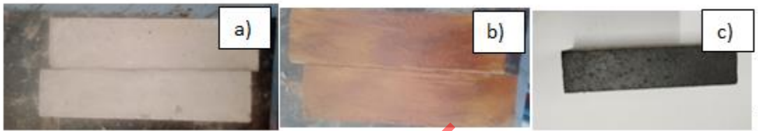
Fig. 4 a, b, c Schematic representation of states of specimen preparation- Plain substrate followed by luminescent covering and finally dark layer covering.
