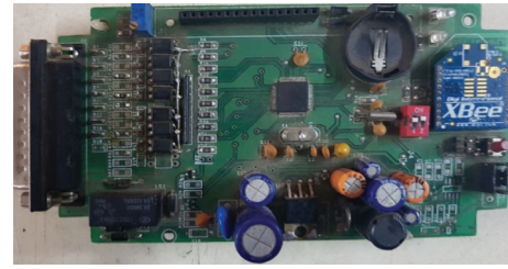
FIGURE 5: Hardware of PIC16f877a with Zigbee.
