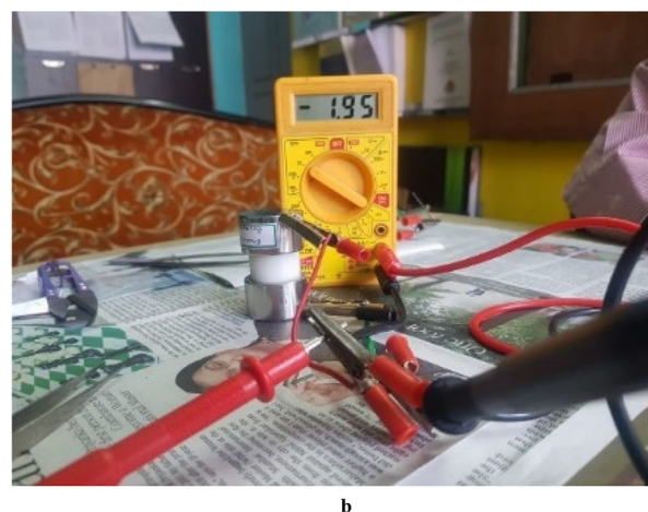
Fig. 19 (a, b) Open-circuit voltage for 0.9 g CSE + 1 g PVA + 0.45 wt% \text{MgCl}_2
