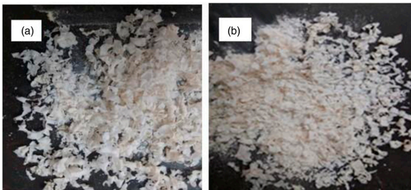
Figure 5. Chip formation during drilling operation in: (a) raw and (b) SB treated fiber composites at 0.166 m/s cutting speed and 0.05 mm/rev feed rate.
