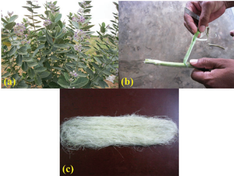
Figure 1. Extraction of CG fiber: (a) CG plant, (b) removal of stem outer layer, and (c) extracted CG fiber.
