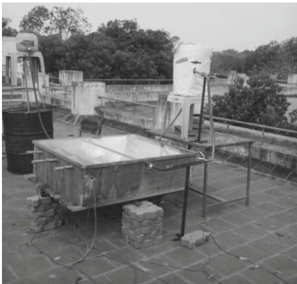
Fig. 4. Experimental view of closed loop setup of PTC.
