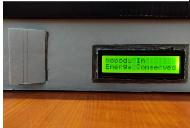
Fig. 8 (b) LCD Display when the count zero
