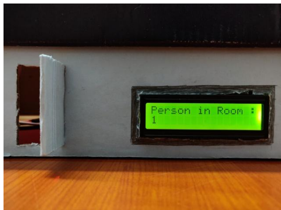
Fig.9 (b) LCD Display, when the count is one
