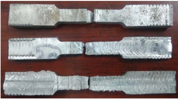
Fig. 8. Fractured surfaces of hybrid composites.
