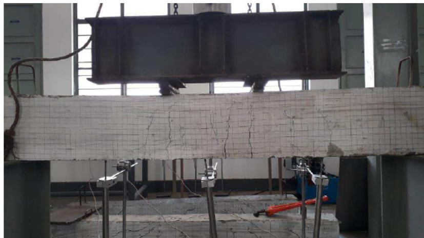
Figure 6 Test setup of a Geogrid beam
