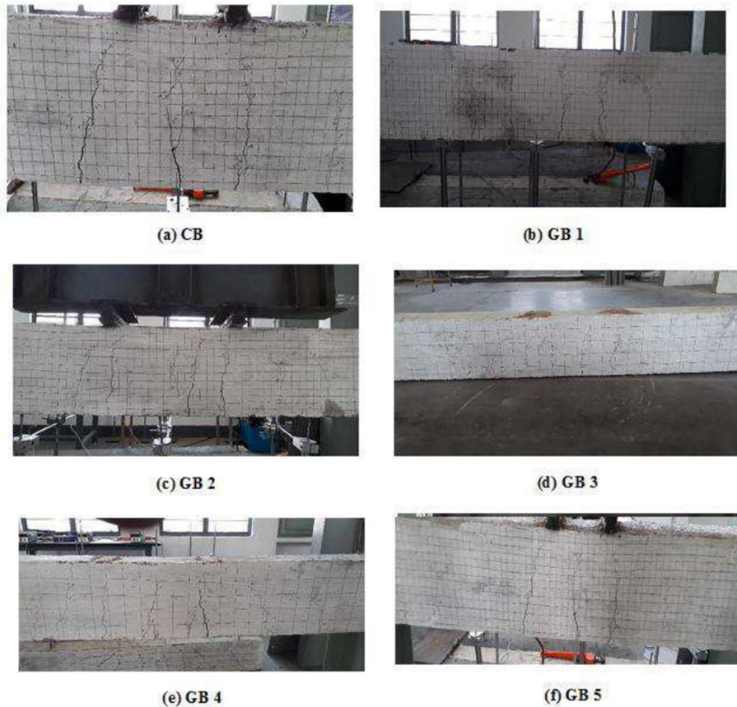
Figure 9 Crack pattern of tested beams
