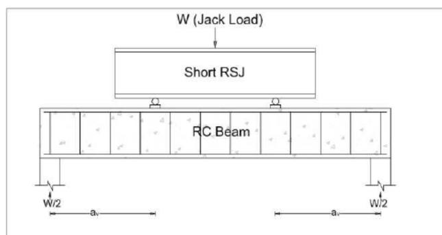
Figure 5 Test setup of a RC beam
