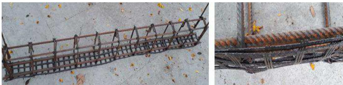
**Figure 3** Geogrid layer as reinforcement
