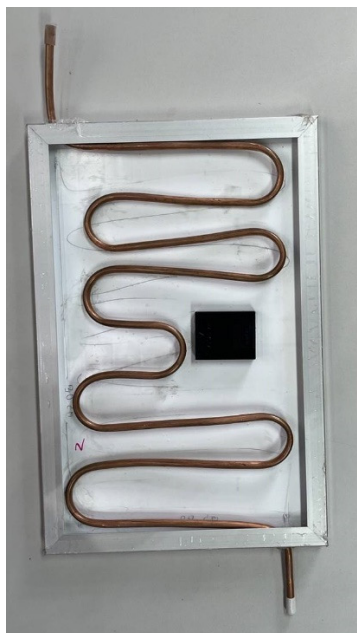
PV with heat transferring pipe
