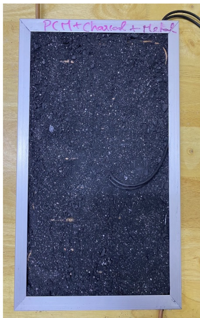
PV with heat transferring pipe and PCM+charcoal+metallflakes
