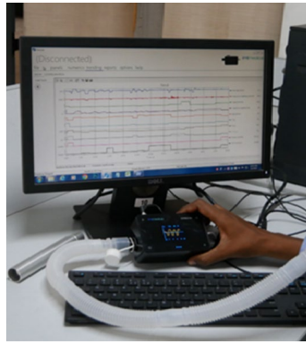
Fig. 8. Experimental setup for capturing the normal breathing pattern.
