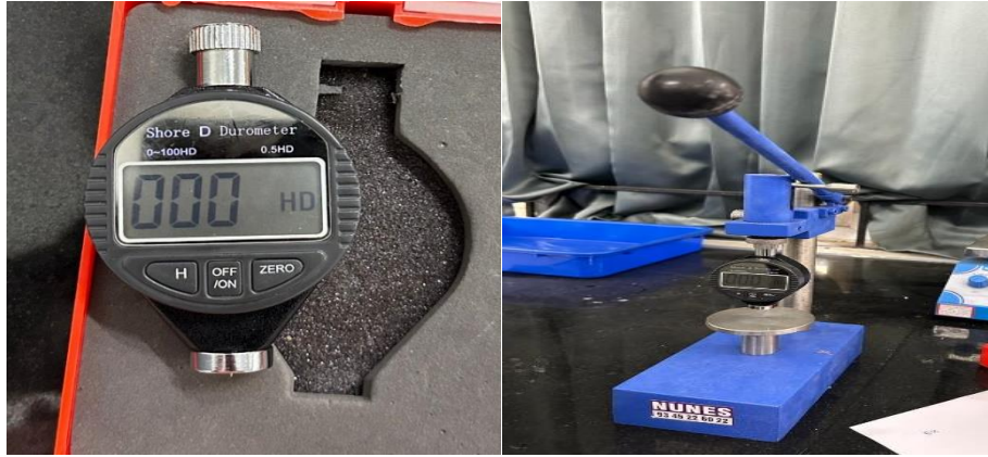
Figure 3: Experimental setup of Shore D hardness Measurement
