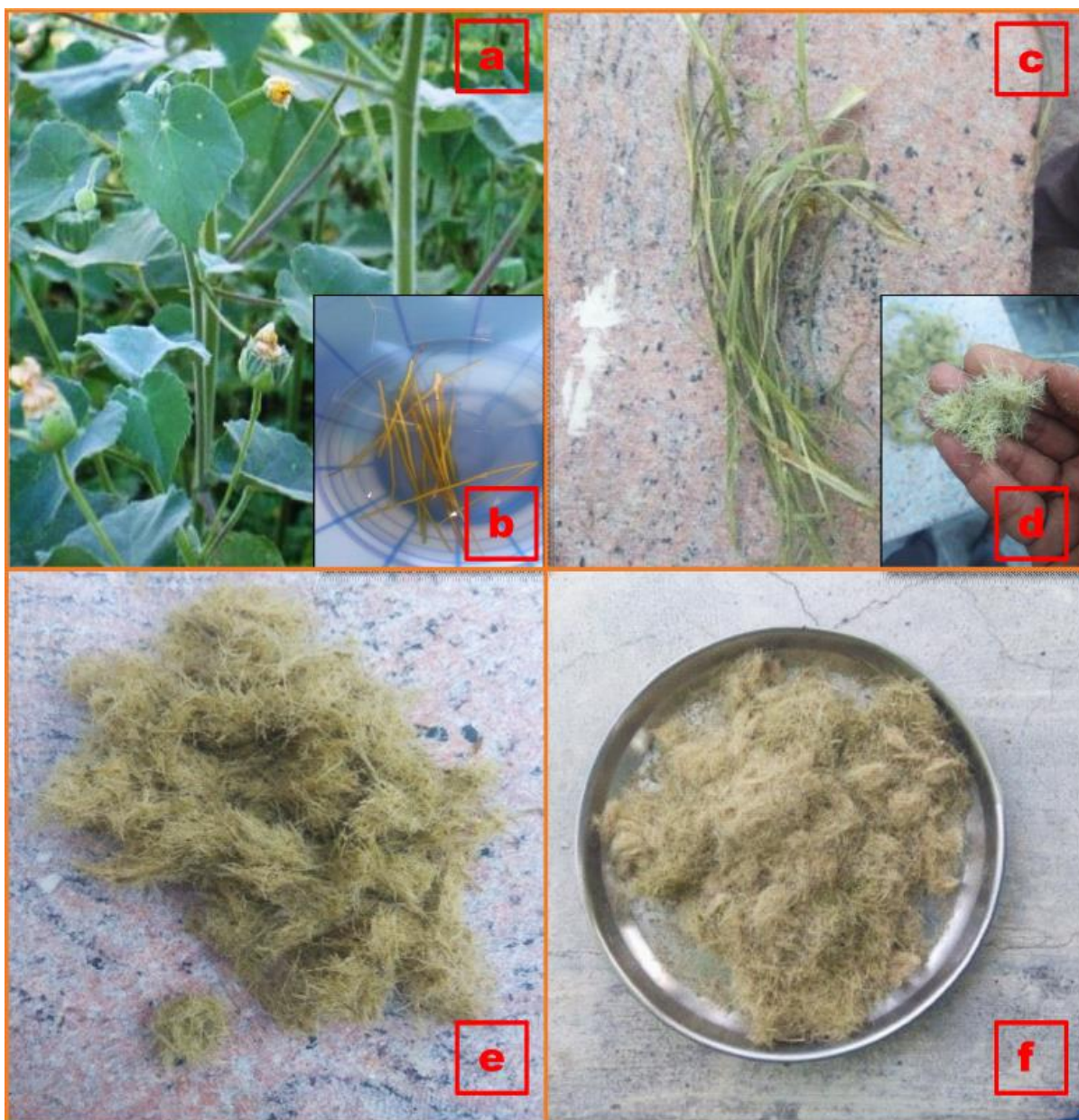
Figure 1: Abutilon Indicum Fiber (AIF) extraction (Reproduced with permission from Wiley, License Number: 5570010817842) [5]
