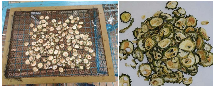
Fig. 5 Quality of the bitter melon while dried by using mixed mode with regenerator and direct sun drying
