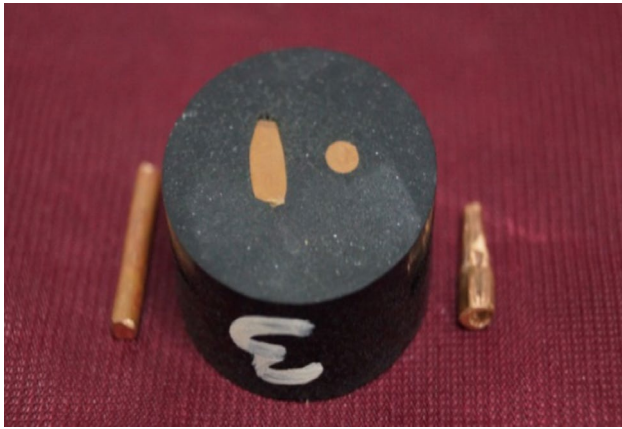
Fig. 12 Copper samples prepared for microhardness testing
