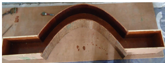
Fig. 3. Fabricated mold for VCRC beam.
