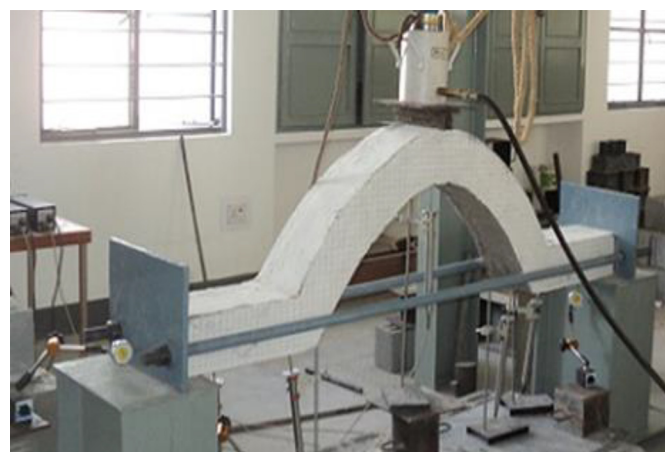
Fig. 4. Testing arrangements of VCRC beam with tie bars.
