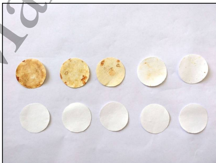
Figure 3.12 Iron chip corrosion test result- MO+2%Cu
