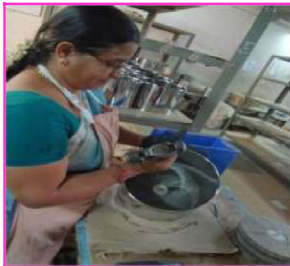
Figure 11 Manual removal of the drum for carrying out rework (see online version for colours)
