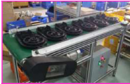
Figure 10 Systematic and continuous feeding of the base frame after implementation of the fourth phase of the CLIM model (see online version for colours)
