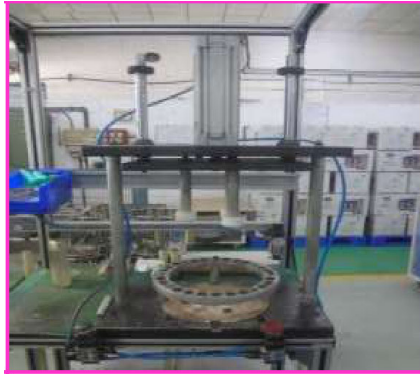
Figure 12 Introduced pneumatic press after the implementation of the fourth phase of the CLIM model (see online version for colours)
