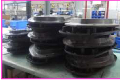
Figure 9 Improper storing and feeding of the base frame (see online version for colours)
