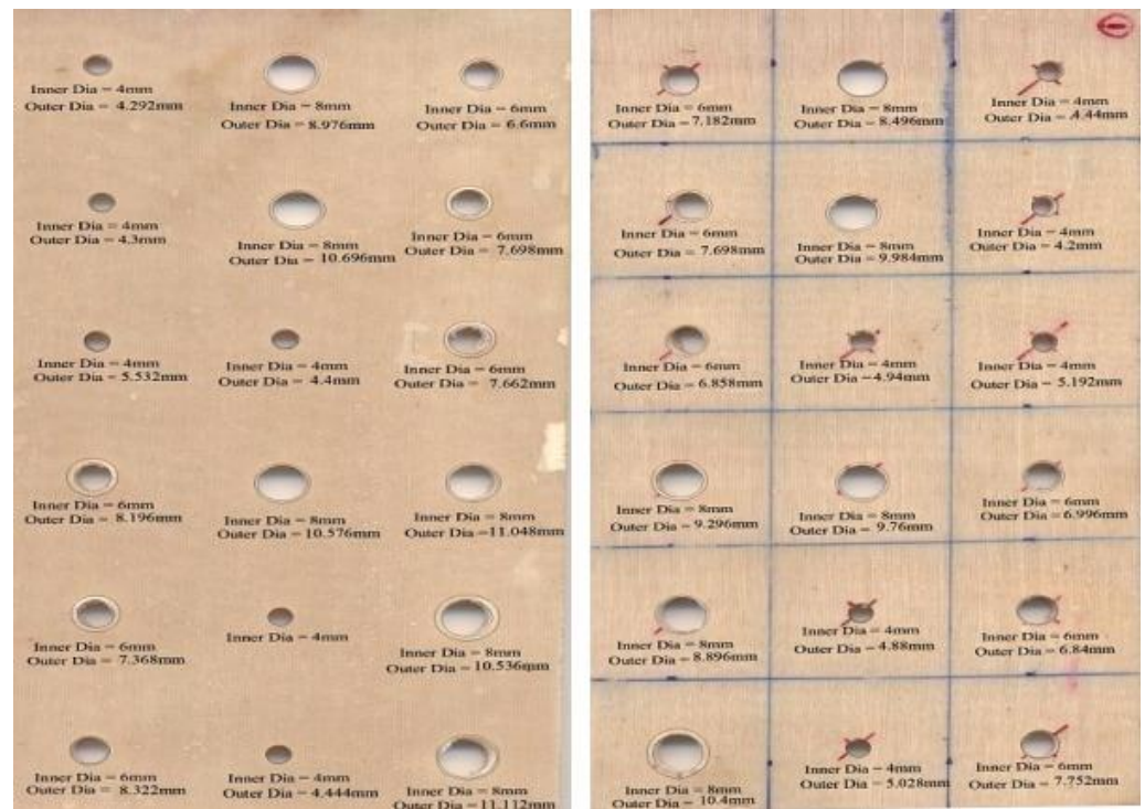
Figure 7. Drilled holes of different diameters and accuracies in bamboo/polyester composites [103].
