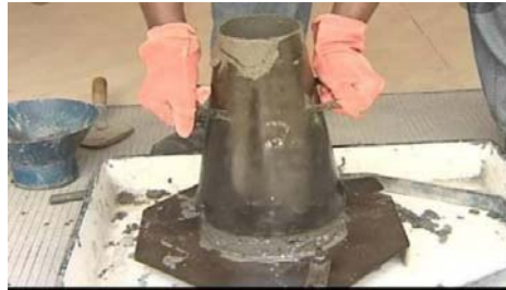
Figure 8. Slump test for workability
