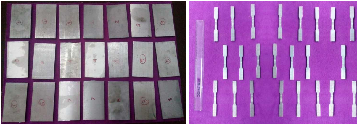
Figure 3. Prepared AMMHC plates for FSW process Figure 4. Tensile strength test samples for FSW joints
