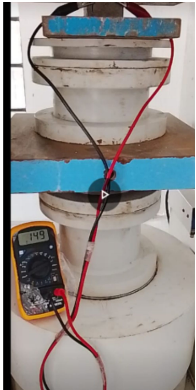
Fig. 10 Voltage output of geopolymer and HAP composite
