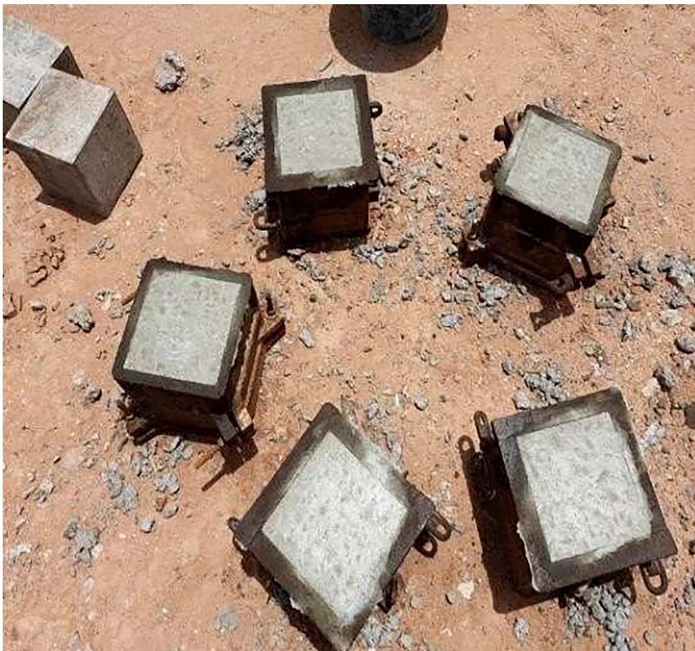
Figure 6: Casting of cube.
