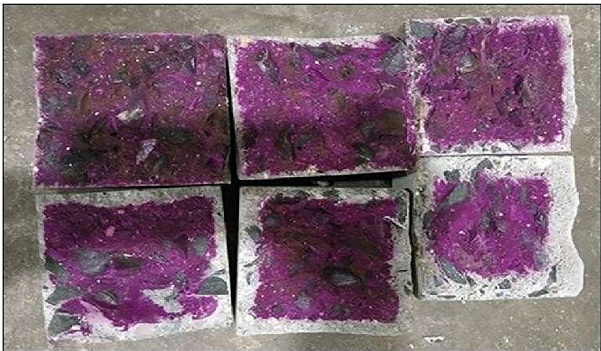
Figure 15: Carbonation depth on cube.
