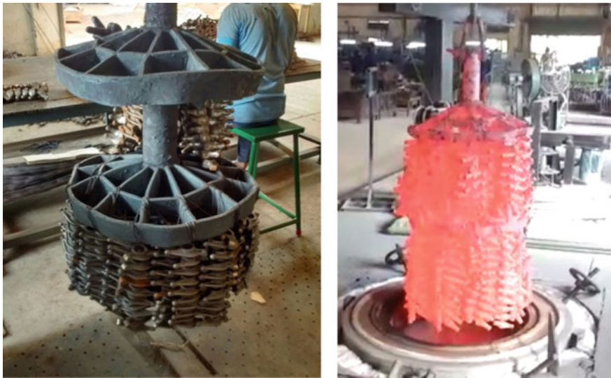
(a) Circular fixture with suspended grey cast iron rocker arm
