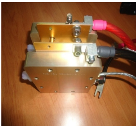
Fig. 1 Assembled Single Cell PEM Fuel cell.
