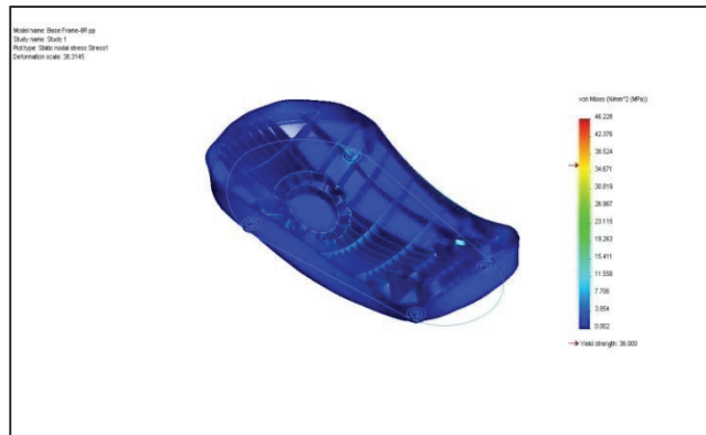
FIGURE 4. Stress Plot of the Existing Back Plate with ABS
