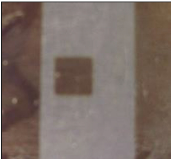
Figure 17. The photograph of negative image obtained from epoxy resin II coated on aluminum plates.
