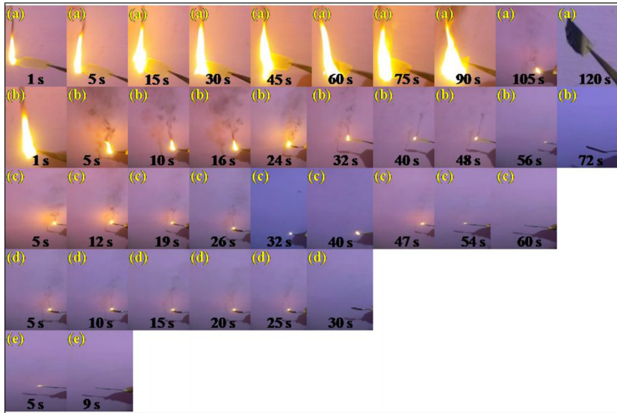
Figure 14. Digital photo images of flame-retardant behaviour of (a) epoxy matrix, (b) SBCBz-EP matrix, (c) 1 wt% HTCP/SBCBz-EP, (d) 3 wt% HTCP/SBCBz-EP and (e) 5 wt% HTCP/SBCBz-EP hybrid composites. SBCBz-EP: siloxane-based cardanol benzoxazine-epoxy; HTCP: hydroxyl-terminated cyclotriphosphazene.
