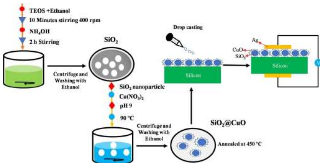
Fig. 1. Schematic diagram of synthesis of \text{SiO}_2@p\text{-CuO} and fabricated \text{SiO}_2@p\text{-CuO}/n\text{-Si} junction diode.
